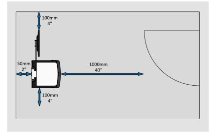
Place the scanner on a level and stable base (at least four table legs). The load-bearing capacity of the base must be suitable for the weight of the scanner (at least 60 kg. / 133 lbs). The dimensions of the base must be suitable for the footprint of the scanner (at least 90 cm x 180 cm /  $36 \times 71$  inch).
