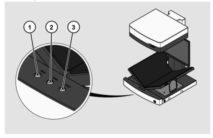
The control panel of the BookTEK<sup>®</sup> 5 V3/V3 Archive/V2/V2 Archive has three buttons with additional functions.
