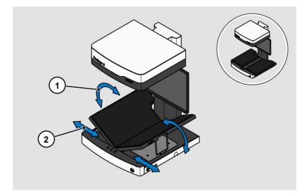
The V position (1) is recommended for very delicate, old books and documents. The opening angle between the book cradle plates is 140 degrees. When the book rockers are lifted into the "V" position, they are held by a support leg on each side. In the "V" position, the plates can also be pushed apart horizontally. The small opening angle puts only minimal strain on the book binding.
