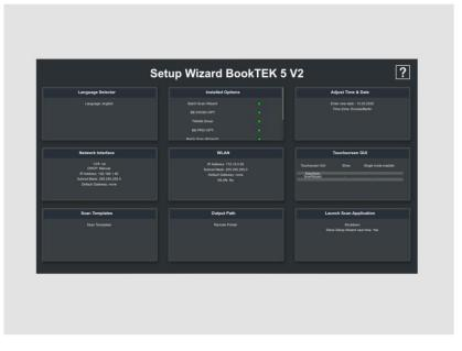
The Setup Wizard allows the user to perform the most important settings on the touch screen during the initial installation of a Scan2Net scanner. After the Setup Wizard has been successfully completed, the scanner can be used immediately without any further settings.
